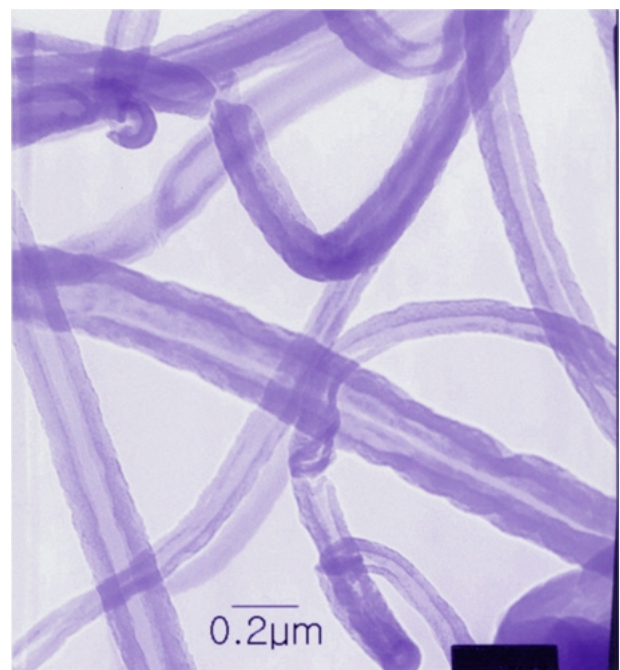
Figure 11 TEM image of PC-MIX electrospun fibers showing an internal rarified core.
